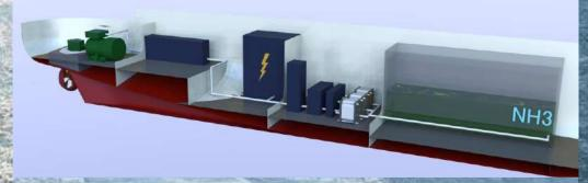
Powered by Fuel Cells using NH₃
